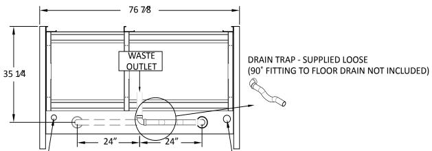
ELECT. STUB OUT\* ALT. FLOOR DRAIN LOCATIONS REFRIG. STUB OUT\*
